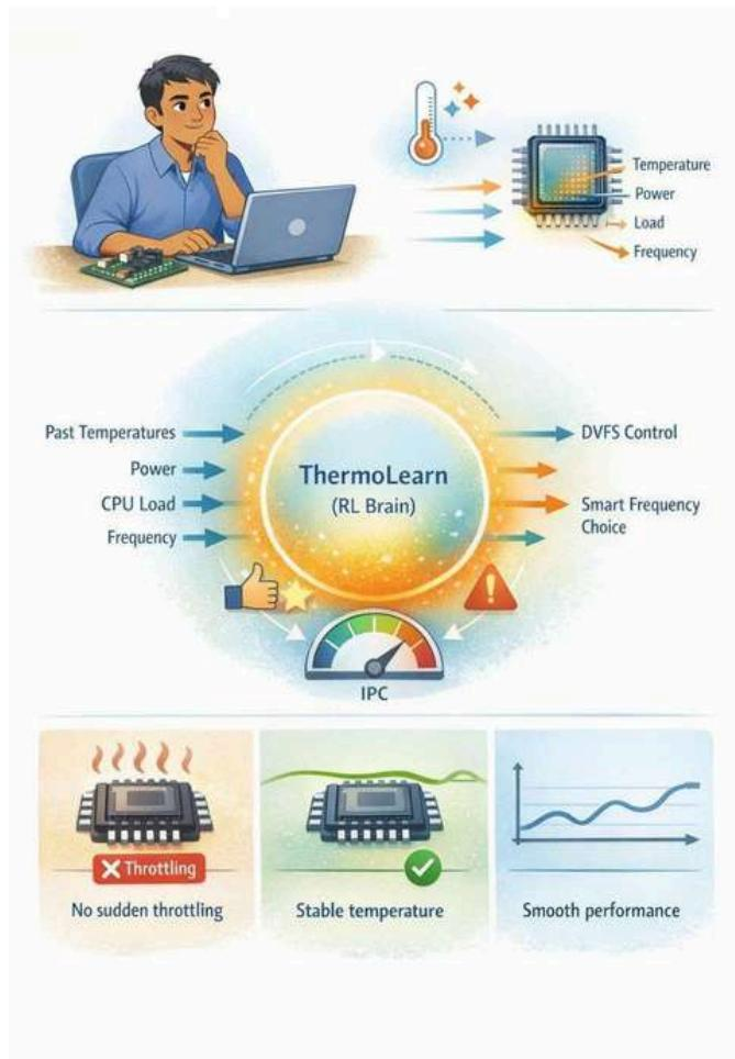
tem forecasts upcoming CPU temperature using past temperature history, power consumption, CPU load, and operating frequency. This predictive ability enables early identification of thermal risk.
